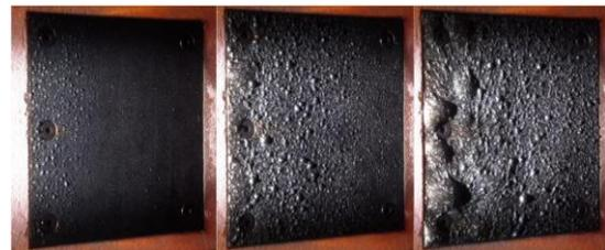
Fig. 10. Bubbles in Aluminium Shear Test
