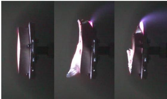
Fig. 8. Failure of Aluminium Top Hat
